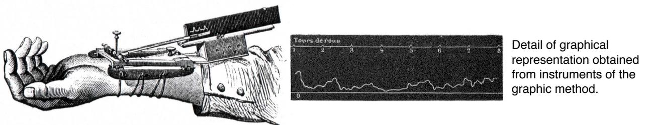
Fig. 1. An illustration of Étienne-Jules Marey's sphygmograph and its resulting trace.
